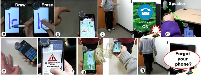
Figure 8 – (a) Left: use pen to draw; Right: use finger to erase; (b) Picking restaurant stored in the off-screen space; (c) Remote gesture to turn on voice mail; (d) Point at a speaker to open a volume controller window; (e) Hand posture for speed-dial; (f) Show a warning message when the user uses the phone behind the wheel; (g) Auto screen rotation based on the proximity to user; (h) Remind the user to take the phone when detects that the user is moving out of the door.
