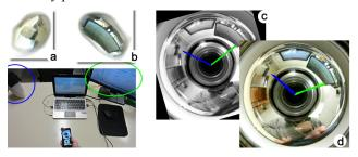
Figure 3 - Reference images: (a) speaker and (b) monitor; (c) rotated input frame for more precise object detection; (d) recognized objects (the blue and green lines indicate the locations of the recognized objects – speaker and monitor).
