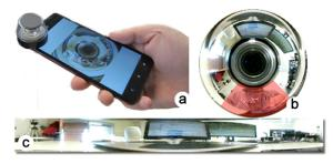
Figure 1 - (a) Surround-See enables peripheral 'sight' on smartphones by means of an omni-directional mirror attached to the mobile device's front facing camera. (b) Surround-See image shows the corresponding scene. (c) The unwrapped image can be used for recognizing the device's peripheral environment (after removing the user's body – shaded in red)
