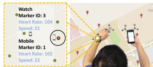
Figure 5. With an External anchor placement, information of markers closest to both devices is shown on the watch.
