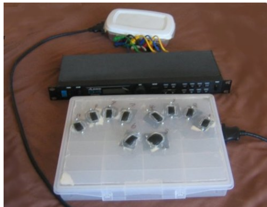
(b) The controller unit connects to the breakout box which connects to a drum module.
